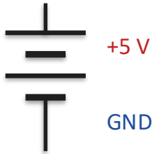
Voltage source the 5 V pin and GND
