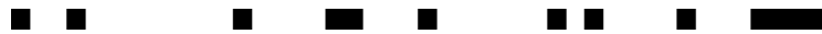
Figure 8.4: Sequence of spots that result when 0 represents a white spot and 1 represents a black spot.
